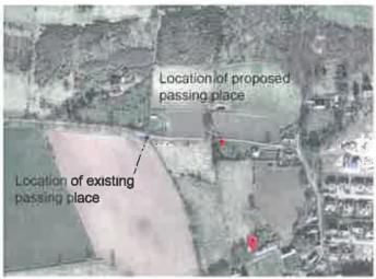
The proposed lay-by/passing place is located at approximately the mid-point of the stretch of road that can be viewed from the top of The Loan and will permit safe passage of vehicles approaching in opposing directions.
